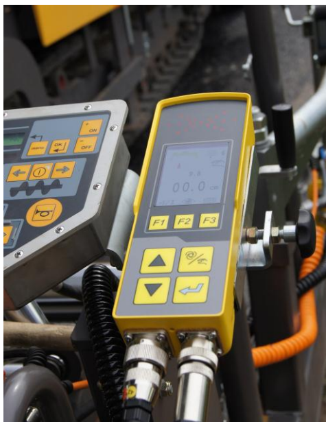
With the MOBA-matic II, the grader operator controls the construction depth and inclination
