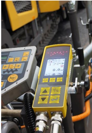
The MOBA-matic II display permanently shows the sensor temperature
