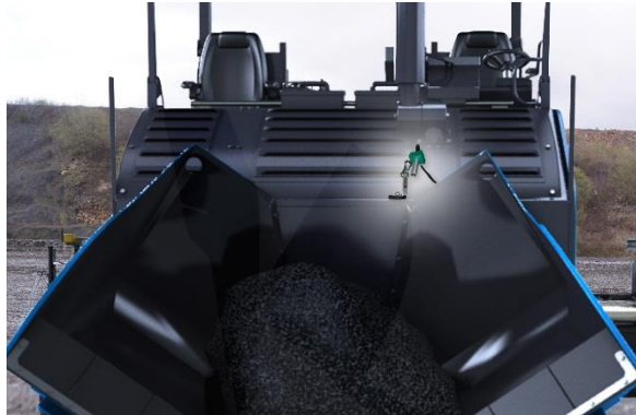
The temperature sensor can be installed either in the hopper or in the area of the screed
